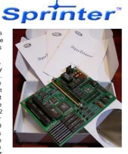
name says, a Logic device that can be programmed at our (read Peters) will. So, we take the Z84C15 (Z80) and transform the Altera into all other ZX Spectrum custom hardware, including the AY chip, and we have a fully working ZX Spectrum out of our Sprinter! Great eh?
